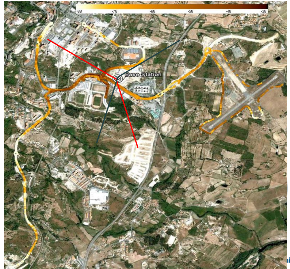
120° sector antenna at 17.15 m
