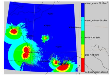
As a second step, study the impact of aeronautical telemetry on MFCN to assess potential QoS
